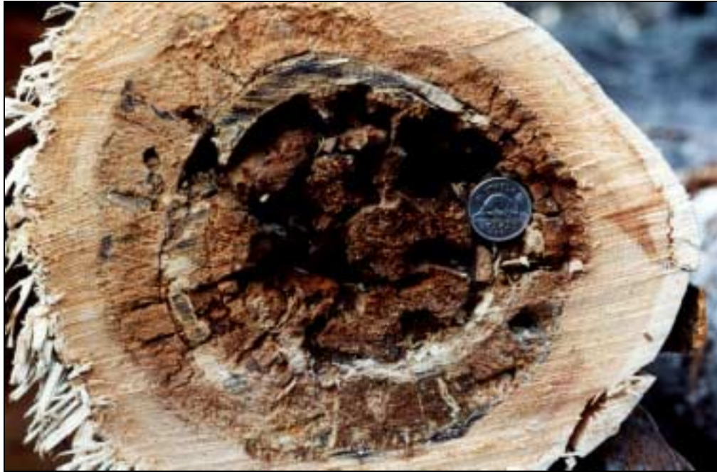
Figure 4.1 Brown cubical butt rot (Phaeolus schweinitzii) in pine.
